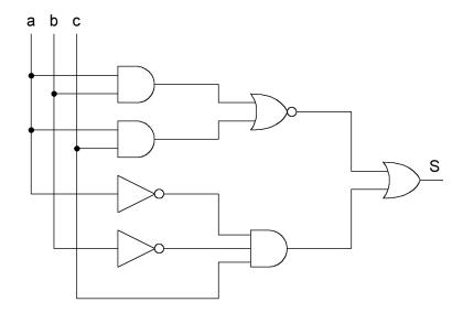
1. Without any simplifications, give the *S* output in terms of *a*, *b* and *c*.
