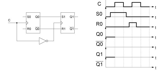
2. Complete the following timing diagrams for a gated RS latch (*Q0*), a positive-edge-triggered RS flip-flop (*Q1*), a negative-edge-triggered RS flip-flop (*Q2*) and a master-slave RS flip-flop (*Q3*).
