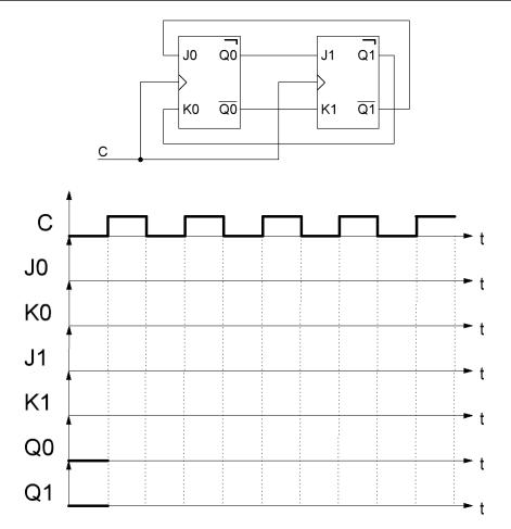
4. Complete the timing diagram for the circuit below.
