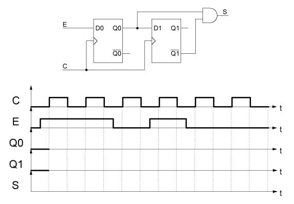
4. Complete the timing diagrams for the circuits below.
