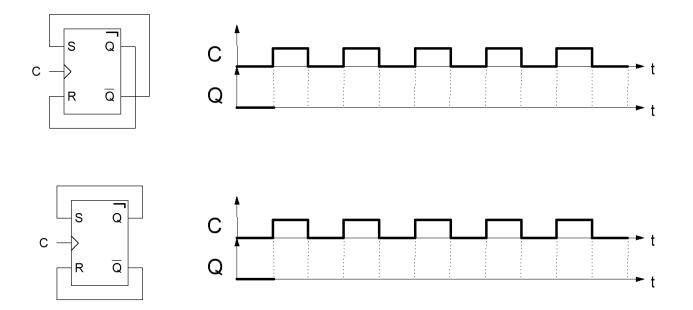
4. Complete the timing diagrams for the circuits below.
