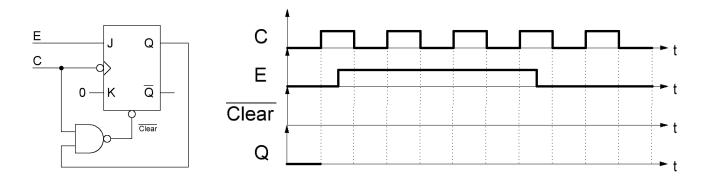
5. Complete the timing diagram for the circuit below.
